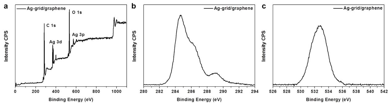
**Fig. S4** XPS spectrum of Ag-grid/graphene on PET substrate. (a) Wide scan of XPS of Ag-grid/graphene on PET substrate. High resolution XPS of (b) C 1s peak and (c) O 1s peak from an Ag-grid/graphene on PET substrate.
