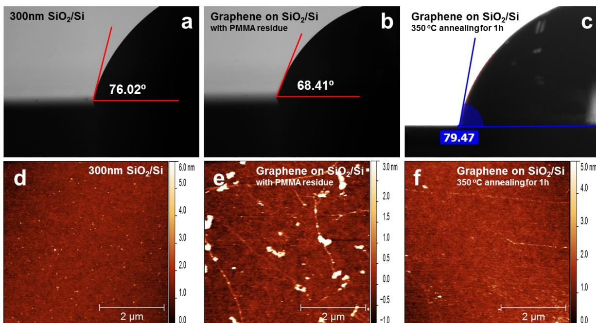
**Fig. S2** (a-c) Contact angles of water droplets on (a) 300 nm  $\text{SiO}_2/\text{Si}$  wafer, (b) graphene after transferred on  $\text{SiO}_2/\text{Si}$ , and (c) graphene/ $\text{SiO}_2/\text{Si}$  after annealing in  $\text{Ar}/\text{H}_2$  at 300 °C. (d-f) AFM
