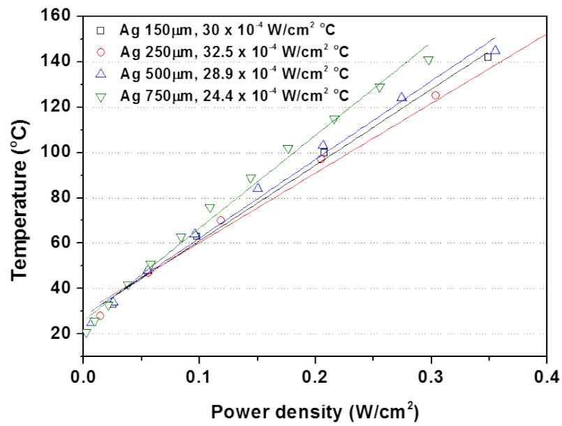
**Fig. S9** Steady-state temperatures of the Ag-grid heaters as a function of input power density.
