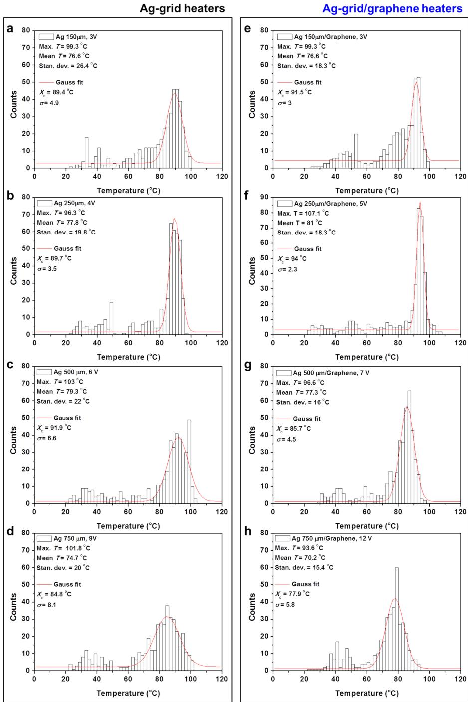
**Fig. S10** Statistical analysis of the temperature distribution in the (a-d) Ag-grid and (e-h) Ag-grid/graphene heaters at approximately 100°C. All data were measured at the steady-state temperatures.
