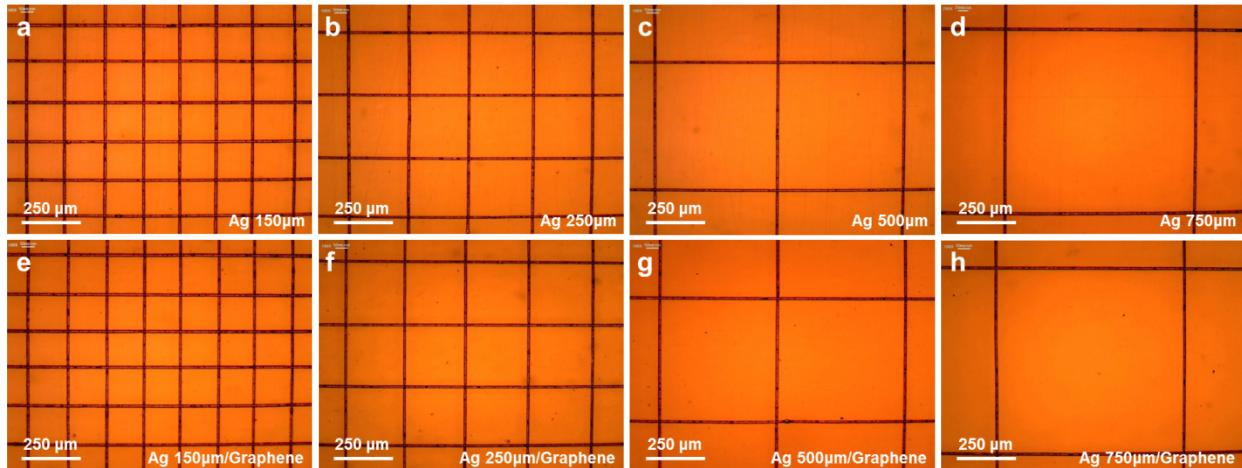
**Fig. S1** The optical microscope images of the square-shaped Ag-grids at different line pitch (150, 250, 500, and 750  $\mu\text{m}$ ) on (a-d) PET and (e-h) graphene/PET substrates. These images are taken under the same magnification.
