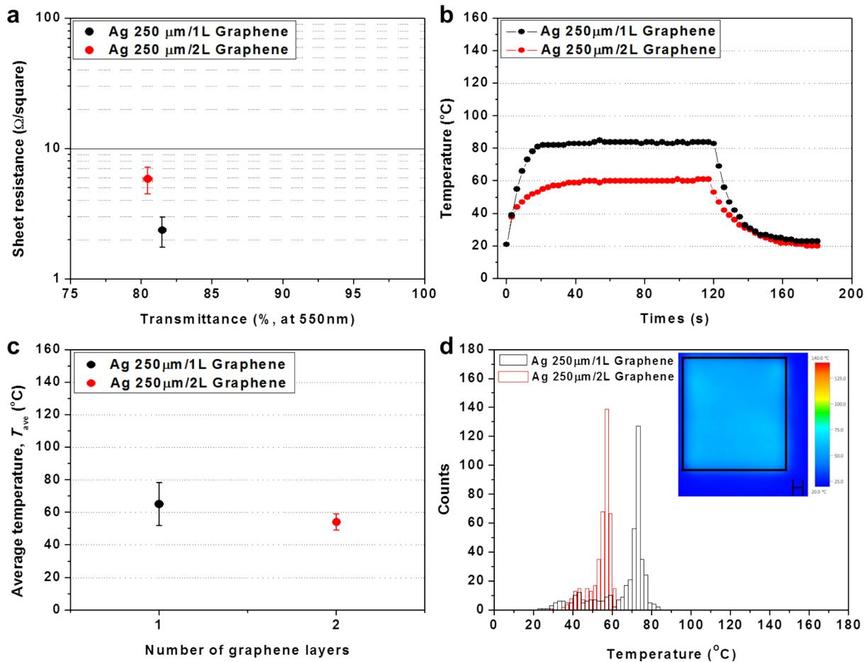
**Fig. S11** Comparison of the Ag-grid/graphene hybrid films depending on the layer numbers of graphene: (a) electrical and optical properties. (b) Time-dependent temperature response. (c) The average temperature and temperature distribution. (d) Statistical analysis of the temperature distribution.
