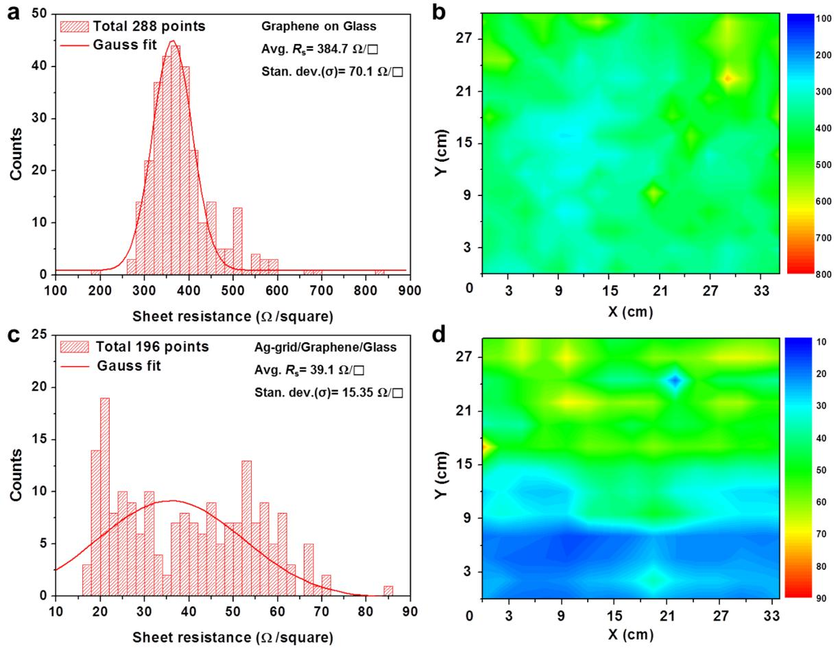
**Fig. S8** Sheet resistance distribution of a large-area (a, b) graphene film and (c, d) a Ag-grid/graphene film on glass substrates. (a, c) The sheet resistance histogram of the  $30 \times 35 \text{ cm}^2$  graphene film and Ag-grid/graphene film. The sheet resistances were measured at 288 points for graphene film and at 196 points for Ag-grid/graphene film. (b, d) The corresponding spatial distribution of sheet resistances.
