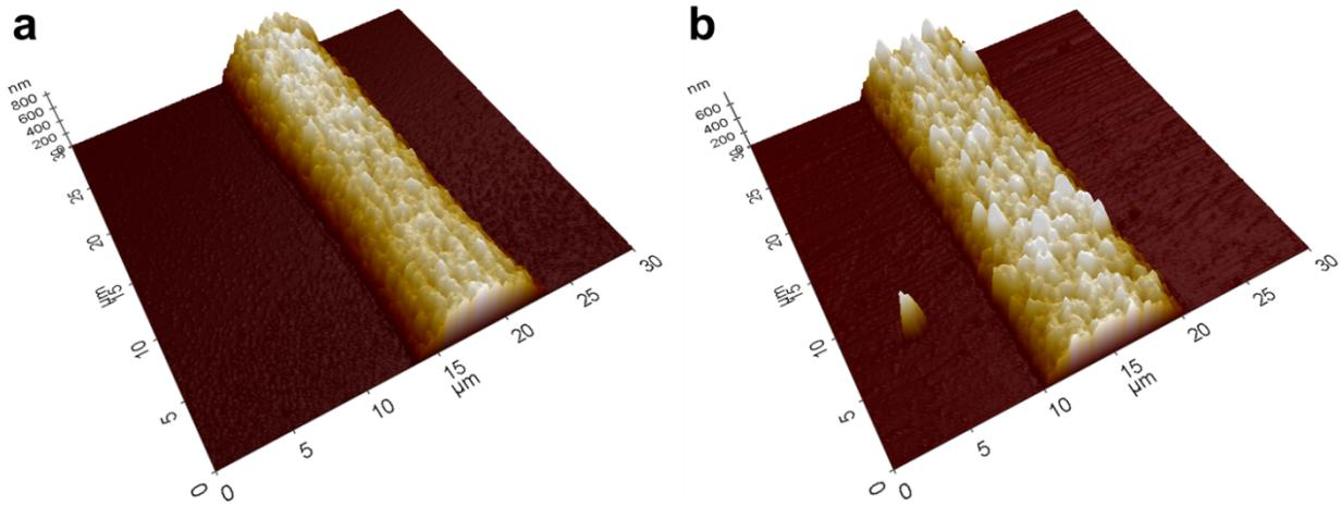
**Fig. S3** 3D profile by AFM images. (a) Ag line and (b) Ag line/graphene on the SiO<sub>2</sub>/Si wafer.
